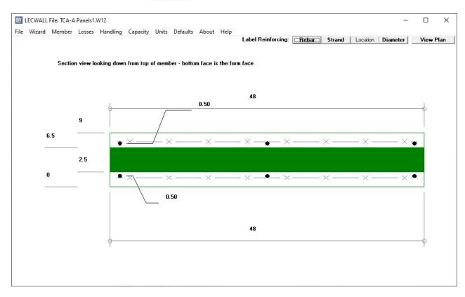
From pg. 98 of the Report, average Fu = 2.82 ksf,  $\Delta u$  = 0.06 in., Ke = 102 k/in,  $\Delta e$  = 0.014 in and Fe = 102\*0.014 = 1.43 ksf. (Generally, the lower-bound values should be used instead of the average, but in this case we are trying to match the test conditions.) The values are per sq ft, so for a default 16" spacing, 5.333 connectors are required in each row (48/5.333\*16 = 144 in2):
