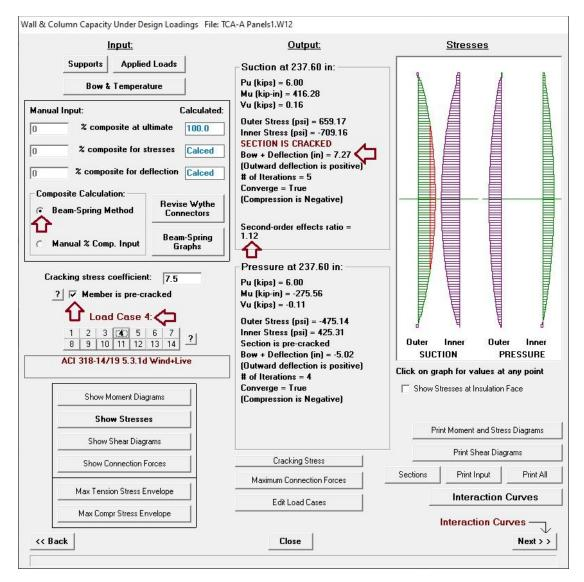
Deflection with P-Delta magnification is 7.27", compared to 5.7" in the TCA report. LECWall applies a Phi-k stiffness factor of 0.875 to EI (per ACI 318). Without that, deflection would be 7.27\*0.875 = 6.36", still greater than 5.7". The *Second-order effects ratio* shows that deflections were magnified 12% by P-Delta effects. ACI limits second-order effects to 40% maximum.
