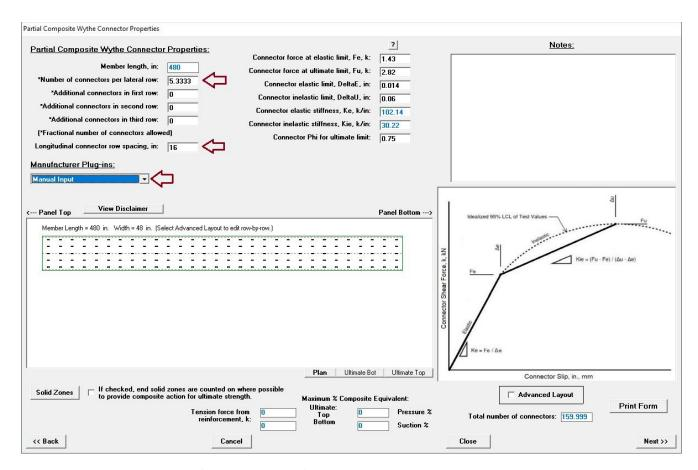
Wind load is applied, 38.75 psf Suction, 25.5 psf Pressure. Any gravity loads should also be applied, but we don't have any, just the panel self-weight, which can still be significant for P-Delta effects.
