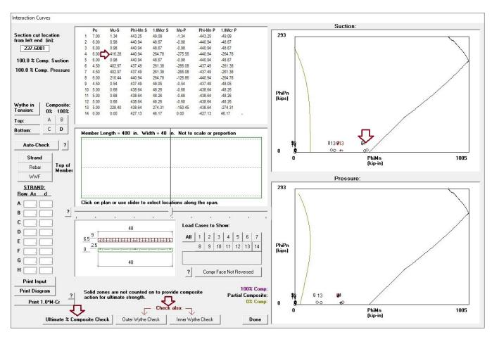
The % Composite check looks ok, but this is misleading, as the individual wythe checks are usually more accurate. Checking the Outer Wythe:
