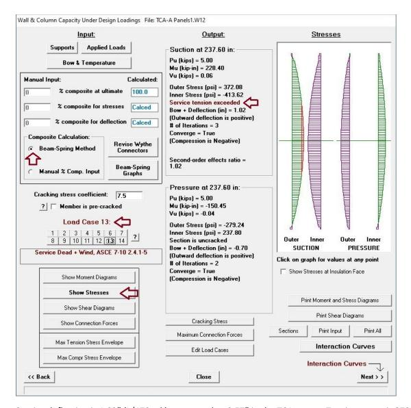
Service deflection is 1.02'' (L/470, ok), compared to 0.57'' in the TCA report. Tension stress is 372 psi (6 SQFC), less than 7.5 SQFC = 461 psi cracking stress, but greater than 5 SQFC = 307 psi, so could be a concern for appearance.
